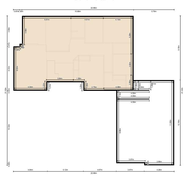
Measurement Diagram for: Basement Exterior Wall Thickness: 17 cm
